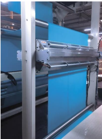
BW Converting's Baldwin TexCoat G4 applies chemistry with pinpoint accuracy — on one or both sides of the fabric — with no contamination, overspray or dilution.
